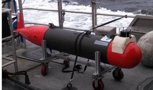
Figure 53. Coastal Glider Rigged with Syntactic Foam Mount for Acoustic Modem
