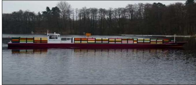
Model of a VLCS with the bridge located at the stern
