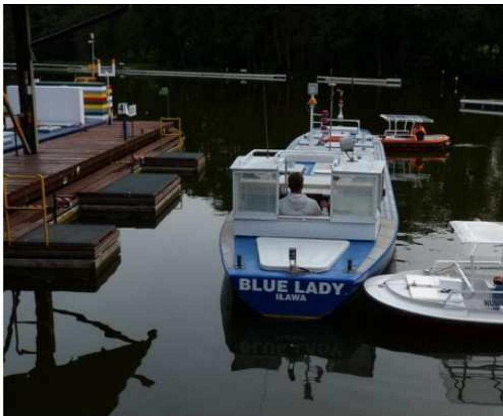
**Two manned models of a large tug built in scale 1:24 pushing a tanker di**
