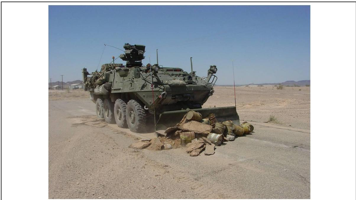
FIGURA 6 - *Obstacle Clearance Blade* removendo escombros
