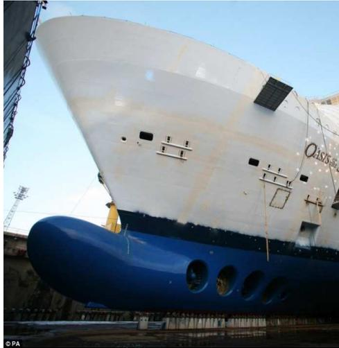
Figura 12 – *Tunnel Thrusters*
