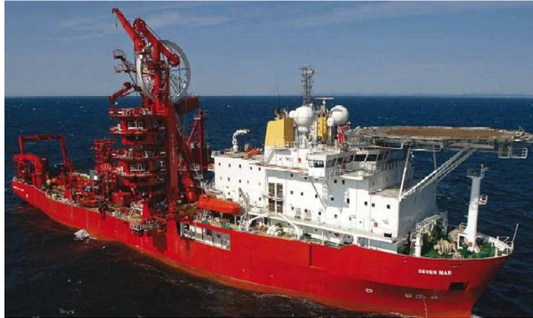
FIG-18 PLSV– Pipe Laying Support Vessel
