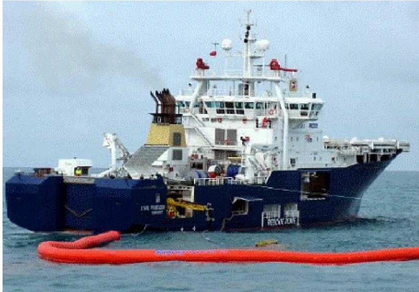
FIG-16 OSRV- Oil Spill Response Vessel
