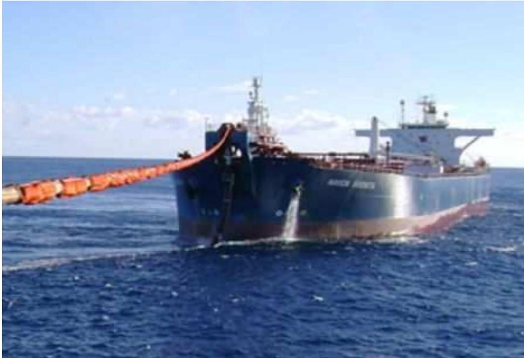
**Figura 17: Shuttle Tanker**
