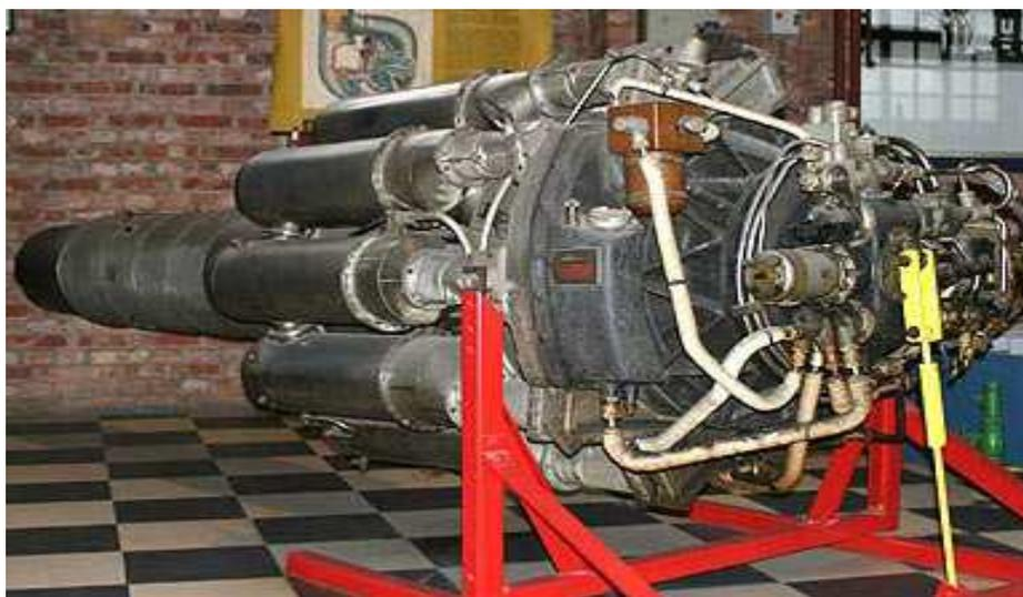
**Figura 6** -Motor do jato do Whittle W2/700.
