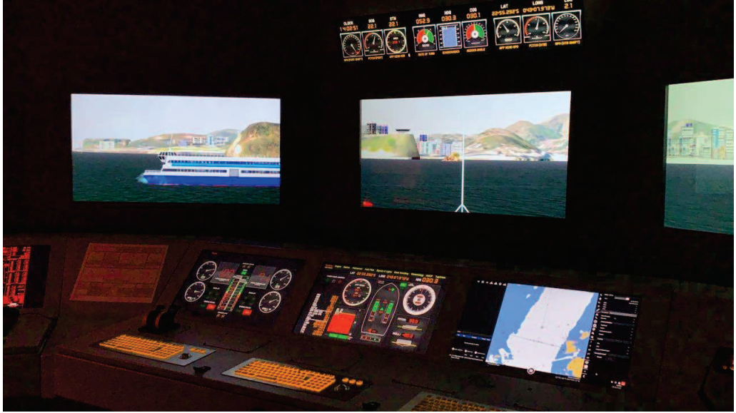
Figura 2.5: Navy Bridge Simulator, used for extracting synthetic images for the proposed classifier.
