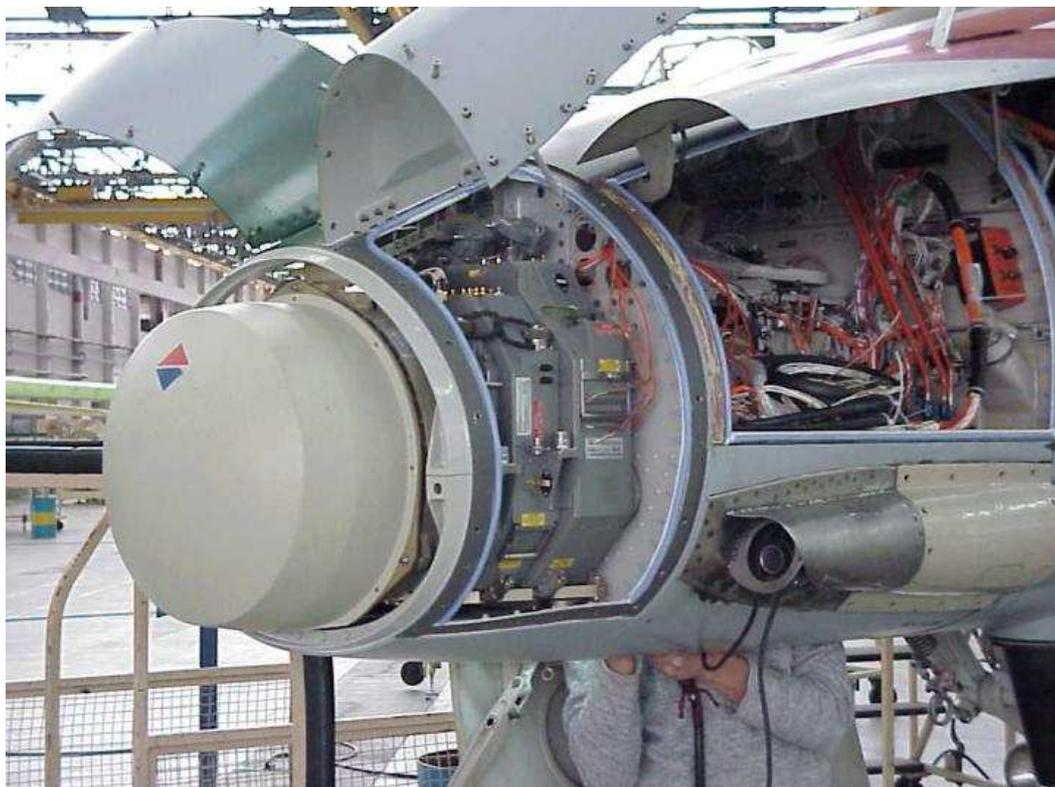
**Figura 21 - Radar SCP-01 (Scipio)**
