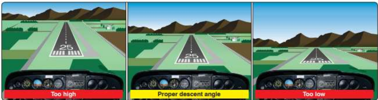
FIGURE 1.1 – Example of visual differences during landing phase. In this case, there are differences in terms of height and descent path angle between images (Extracted from Federal Aviation Administration (2016)).
