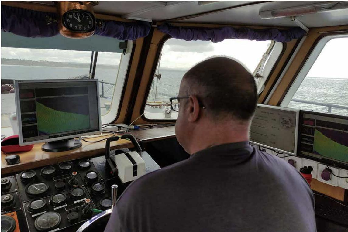
**Figure 3 Interior of the hydrographic small boat carrying out multibeam surveying (Instituto Hidrografico).**
