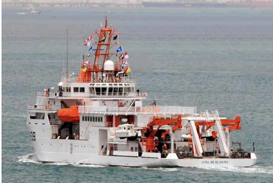
**Figure 1 Hydroceanographic Research Vessel “Vital de Oliveira” can conduct hydrographic surveys with its two hydrographic research boats and an ROV (Brazilian Navy).**
